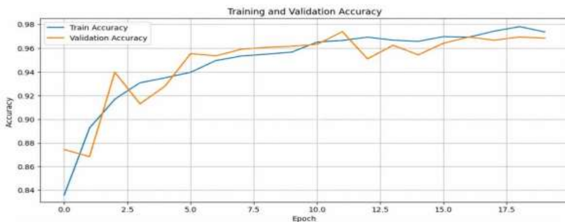
Figure 8. Training and Validation Curves of DenseNet201. Accuracy (left) and losses (right) by each era of training.
